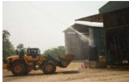
Rain Water Gun at Crushers Charging Platform
